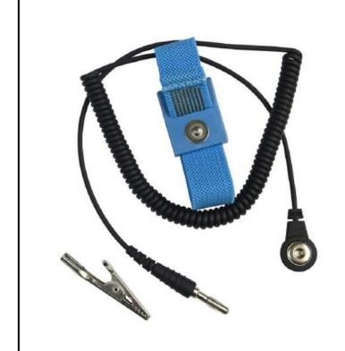
This SCS Economy Single-Wire Adjustable Wrist Strap set provides a cost-effective means of grounding production employees. This wrist strap features an adjustable fabric wristband with a 6-foot retractable coil cord, alligator clip and a 4mm snap. Meets ANSI/ESD S20.20 and ANSI/ESD S1.1.
